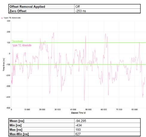
Figure 19. 1 PPS absolute time error under multipath conditions
