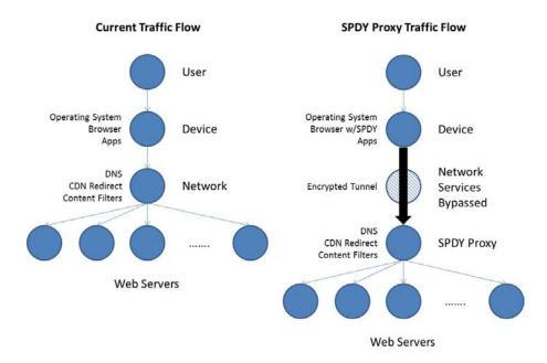
Figure 1: SPDY-based Proxy Traffic Flow
