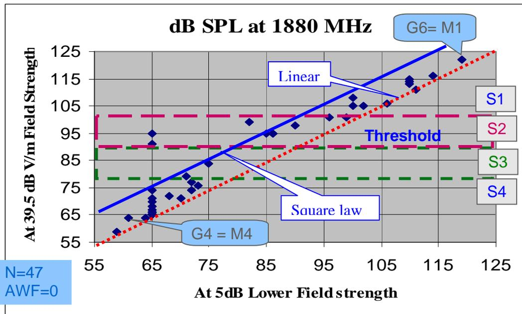
Based on the C63.19 square law assumption, two 10 dB wide SPL bands (marked S2 and S3) are incorporated in the preceding graphs that may correspond roughly to the two 5 dB wide RF level bands, based on the two HAs that were measured per C63.19, that establish rough endpoints to be positioned on the graphs for an estimate of the location of the FCC RF acceptance threshold defined as the boundary between M2 and M3.
