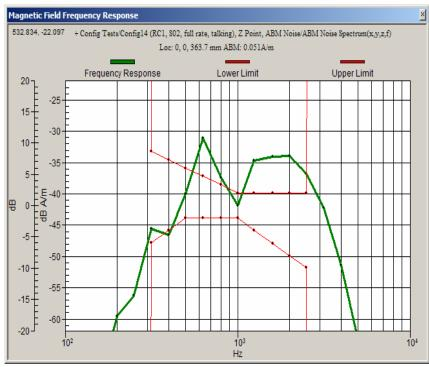
RC1, SO2, vocoder rate full, talking near the phone platform while the ABM2 measurement is being made.
