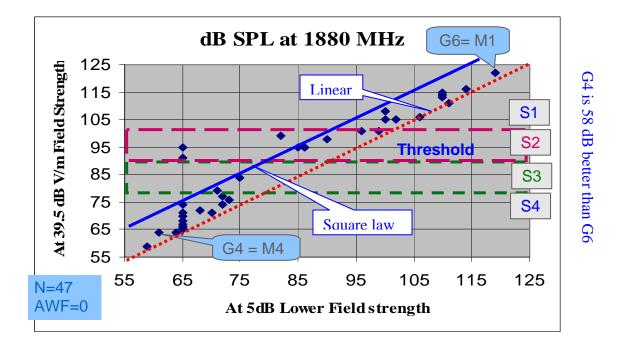
Based on the C63.19 square law assumption, two 10 dB wide SPL bands (marked S2 and S3) are incorporated in the preceding graphs that may correspond roughly to the two 5 dB wide RF level bands, based on the two HAs that were measured per C63.19, that establish rough endpoints to be positioned on the graphs for an estimate of the location of the FCC RF acceptance threshold defined as the boundary between M2 and M3.
